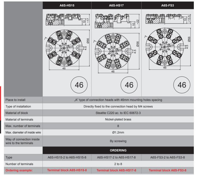
Unit for fixing to the connection head
